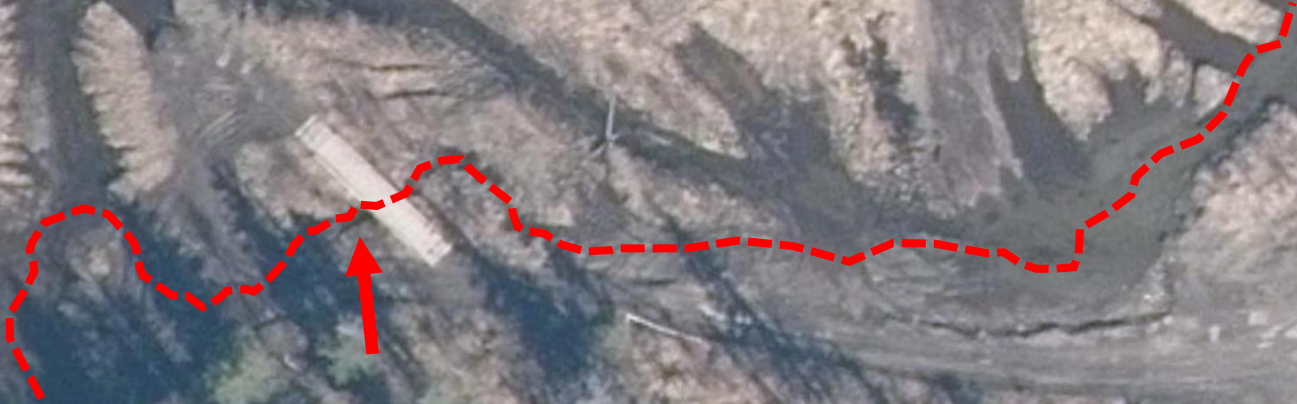
Entrenched and overwidened channel – Channel captured by vehicle track
