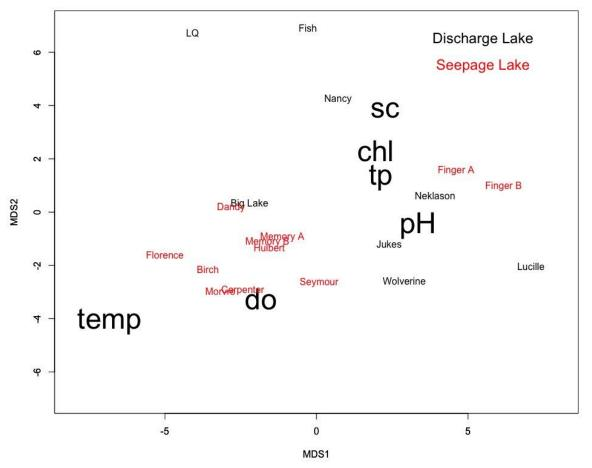
sc – Specific Conductivity chl – Chlorophyll-a tp – Total Phosphorus pH – pH do – Dissolved Oxygen temp – Temperature
