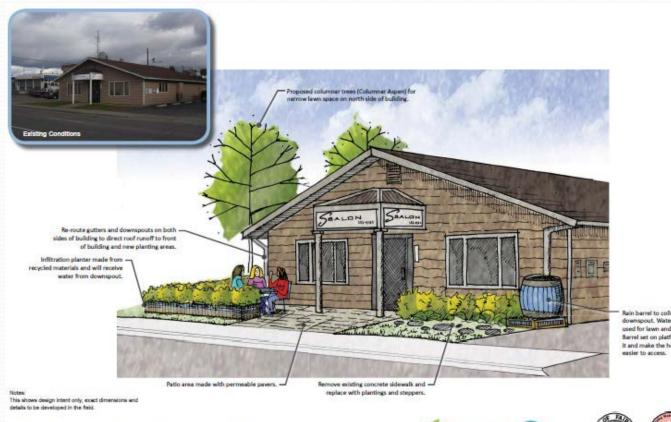
Rain barrel to collect water from downspout. Water collected to be used for lawn and new plantings. Barrel set on platform to protect it and make the hose connection
