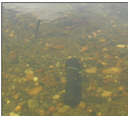
Example of deployment method with data logger inside PVC housing and secured by a cable to rebar.
