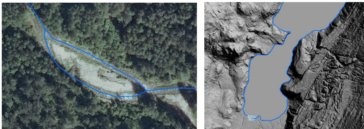
Figure 2. Example of using imagery (left) and bare earth DEM (right) for heads up digitizing
